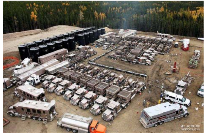
Source: Trican frac job, Canada, as shown in Icon Energy march quarter 2011 report
